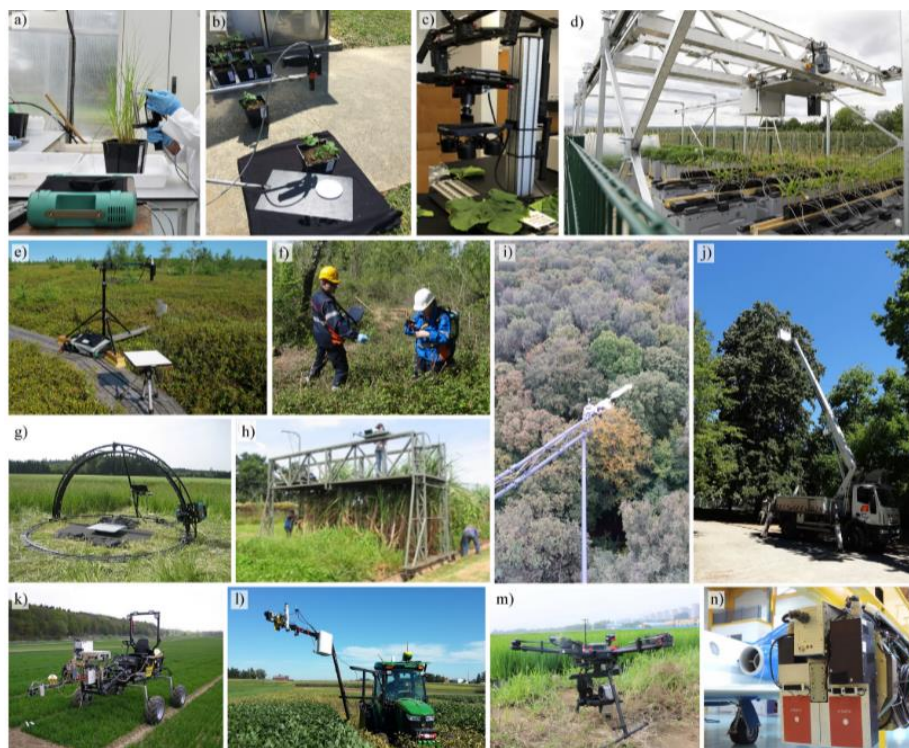
Figure 2. Various proximal sensing platforms for spectral data collections (a) leaf reflectance using a leaf-clip attached to a spectroradiometer, (b) canopy reflectance using a fore optics fixed at nadir, (c–d) close-range hyperspectral imaging of (c) leaf samples and (d) plants, (e–h) canopy reflectance in the field using a spectroradiometer (e) a fixed at nadir, (f) handled, and (g) mounted on a goniometer system and (h) a mobile platform, (i–j) tree canopy reflectance using (i) a tower and (j) a telescopic boom lift, (k–l) canopy reflectance using a spectroradiometer mounted on (k) a motorized vehicle and (l) a tractor. (m) Drone- and (n) airborne-embedded hyperspectral imaging spectrometers proximal and images. (Lassalle, 2021)
